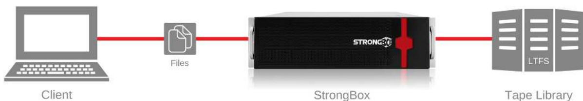
Files written to StrongBox are migrated to tape using Linear Tape File System (LTFS) technology. LTFS enables tape to be mounted as a file system independent of the underlying operating system. This relieves tape of its age-long dependency on backup applications and other proprietary software to store and retrieve data. Because StrongBox is a file-based online archive system, data is continuously available for reading and retrieval in an open, non-proprietary and fully portable format.
